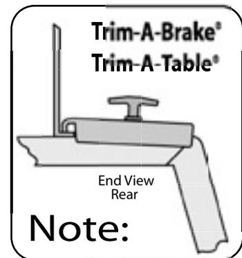
For use with either Trim-A-Brake or Trim-A-Table, insert front lip as described in Step 3. Next, position latch plate horizontally over mounting surface with tab over the lip of the rear rail. Secure in place with "T" knobs.
