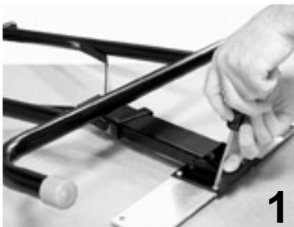
Using the sheet metal screws provided, attach mounting plates to leg strut flanges as shown. Turn brake over and rest each leg assembly onto base rails with the mounting plates extending toward center of brake.
