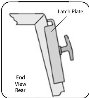
Locate latch plates and position to end assemblies as shown above. For now, loosely thread "T" knobs through slots and into end assemblies allowing plates to remain below the mounting surfaces.
